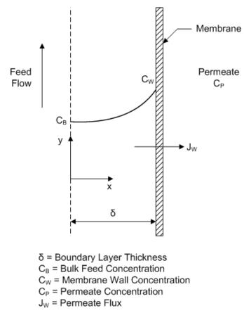
Concentration Polarization = C<sub>W</sub>/C<sub>B</sub>
