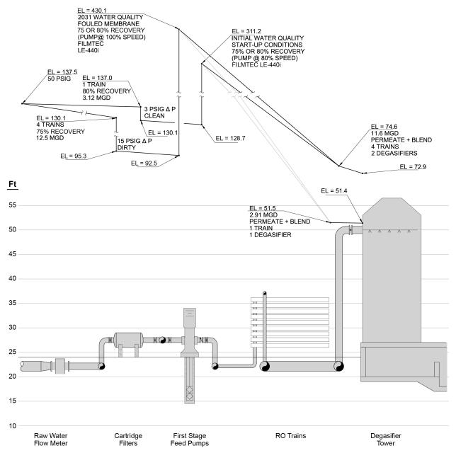
Figure 4-3. Example 1 hydraulic profile – membrane feed and permeate.
