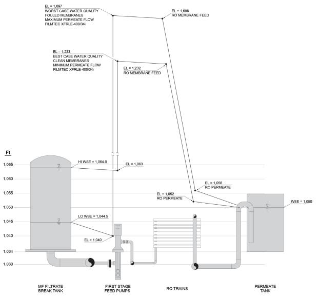
Figure 4-8. Example 2 hydraulic profile.
