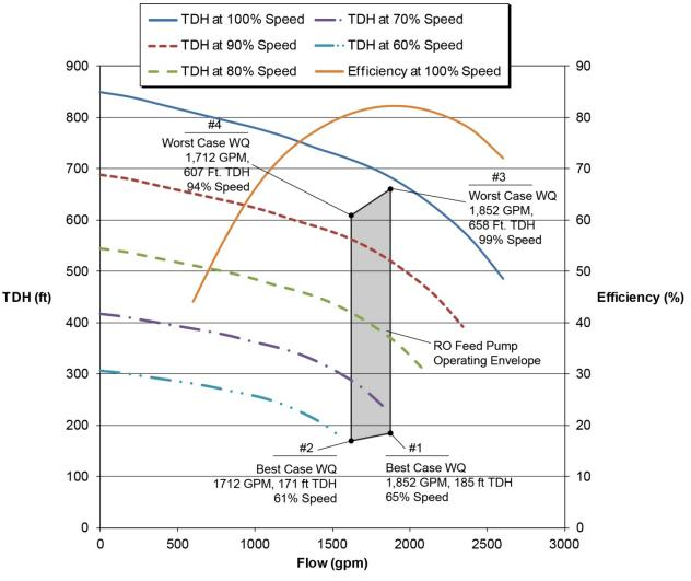
Figure 4-9. Reverse osmosis feed pump operating envelope.
