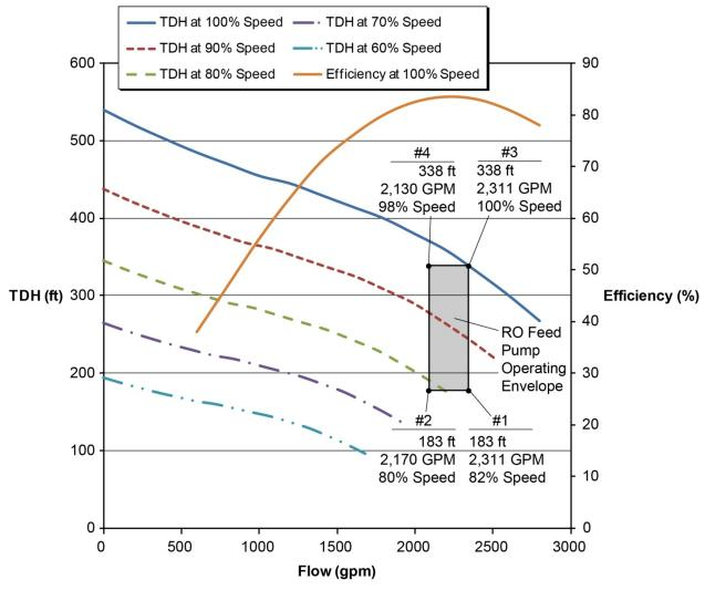
Figure 4-4. Example 1 - reverse osmosis feed pump operating envelope.
