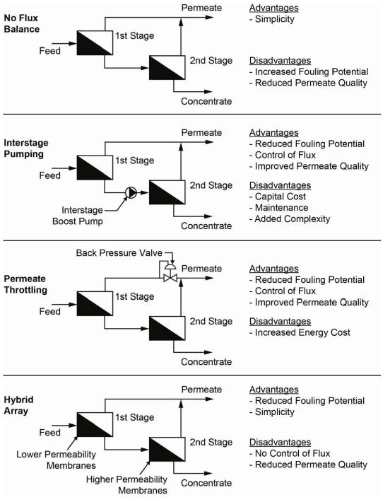
Figure 3-6. Flux balancing alternatives.
