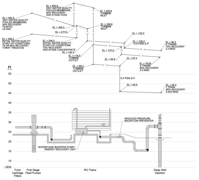
Figure 3-4. Sample hydraulic profile – membrane concentrate.
