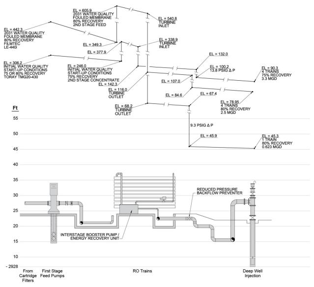
Figure 4-5. Example 1 hydraulic profile - membrane concentrate.
